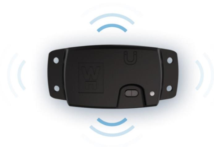
The contractor installed 22 waste container filling sensors in two densely populated parts of the city in 6 locations. Due to the fact that the city of Kežmarok does not have coverage of the IoT network, the sensors were connected via the GSM network, which is demanding on the battery life of the sensor and some functions of the sensors were suspended.
